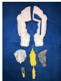
Figure 3: Nasopharyngeal airway mold 3D printed in PLA
